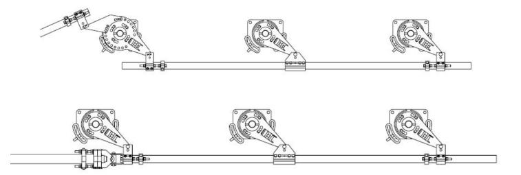
a. With the interphase pipe centered and all clevises in place, pierce the interphase pipe with at the locations shown. Do not remove plastic caps at this time.
