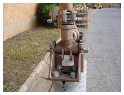
Figure 7: Typical Operating Mechanism
