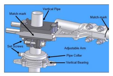
Figure 10: Typical Operating Arrangement
