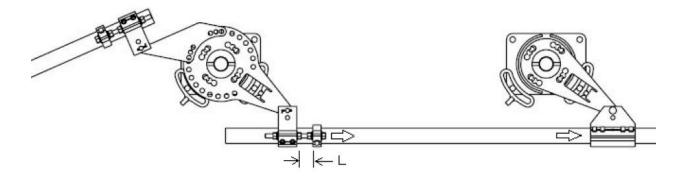
c. Set the timing of the last phase by adjusting the length "L" of the Rapid-Set clevis attached to the last phase.
